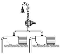
Connection of two pumps with a total input not exceeding 1.5 kW (2 HP).
