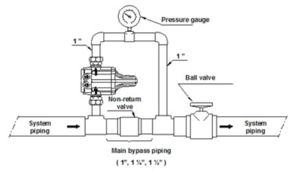
In the event of the pressure losses caused by the installation of the PRESSCONTROL taking the system flow rate down below the desired value, it is possible to install the PRESSCONTROL in bypass as indicated in the figure .
