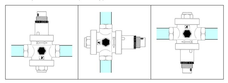
Pressure reducing valves can be damaged by dirty water; therefore we advise to install a self-cleaning filter upstream before the pressure reducer, in order to protect the valve and any other mechanism downstream (thermostatic mixers, taps, etc.).
